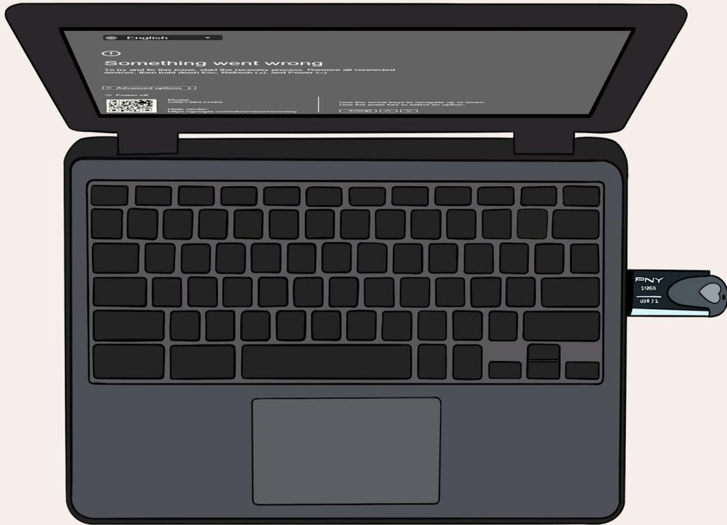
Once you plug in the USB or SD card with the recovery image, press and hold 'Escape' key.
